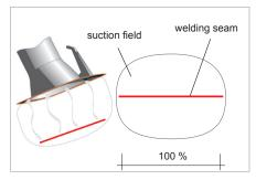
KEMPER exhaust hood with flangeshaped overlep
