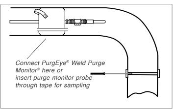
Alternatively, the monitor can be used in the sampling mode. The stainless steel probe is inserted either into the volume being purged or the exhaust port. The rubber bulb is then used to draw a sample of the gas across the sensor.
